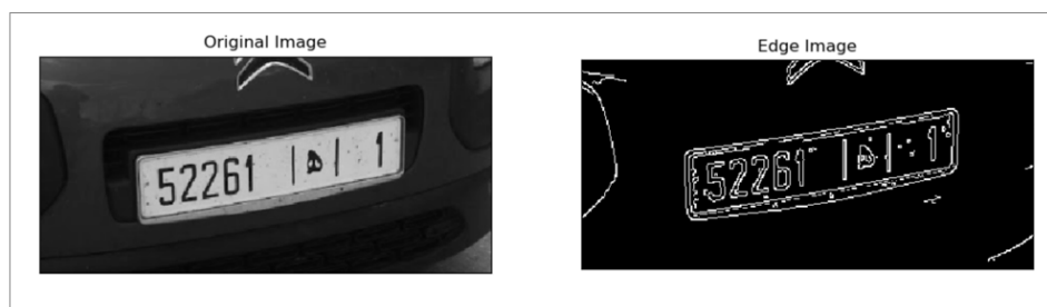
Figure 11: Canny Edge Detector applied on license plate image with two threshold values: 50, 100.
