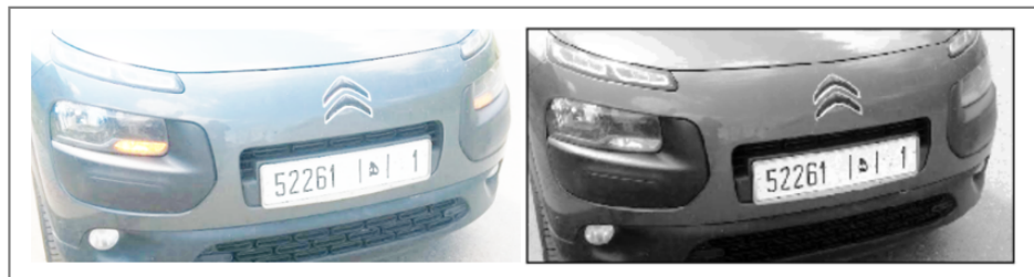
Figure 5: Histogram Equalization used in an input image with low contrast on left.
