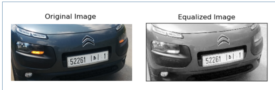
Figure 3: Original Image on left before applying Histogram Equalization, Pre-processed Image by HE on right.
