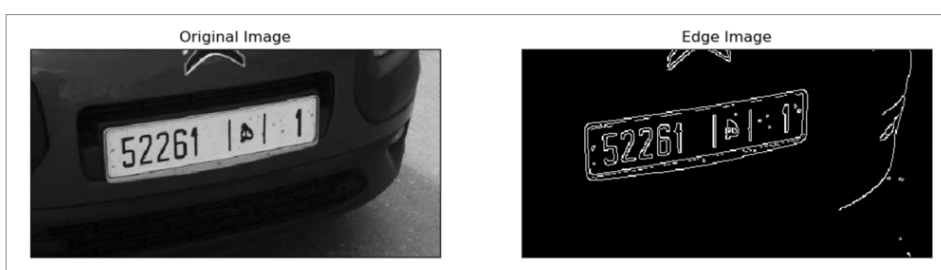
Figure 13: Canny Edge Detector applied on license plate image with two threshold values: 100, 200.
