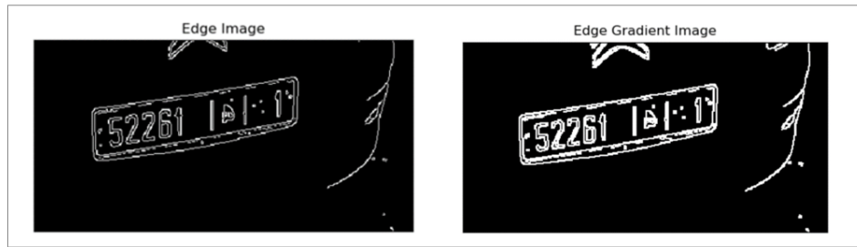
Figure 14: Morphological Gradient Transformation applied on the Canny Edge Detector Method.
