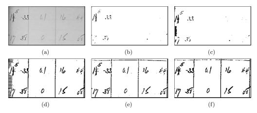
Fig. 4. A fragment of a logbook (a) processed with: (b) Otsu's global method; (c) Otsu's local method based on image partitioning; (d) moving averages,  $n=20,\ s=0.95$ ; (e) Sauvola's method,  $9\times 9$  structuring element,  $R=128,\ s=0.05$ ; (f) the proposed algorithm,  $n=20,\ R=128,\ s=0.05$
