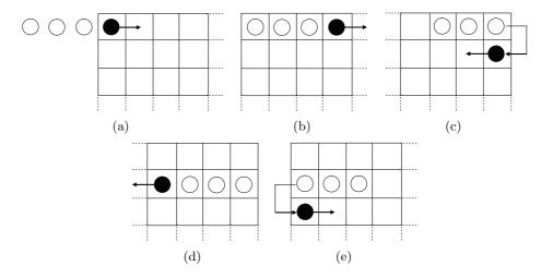
Fig. 2. The pixels of the image as squares and the structuring element of the onedimensional filter as circles, where the blackened circle is the element of the filter, which lies on the pixel currently processed
