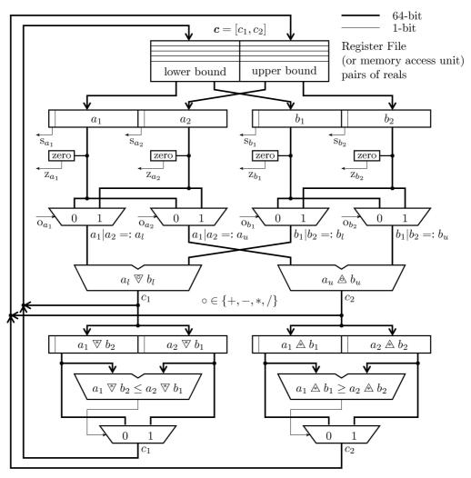
operands:  $\boldsymbol{a} = [a_1, a_2], \ \boldsymbol{b} = [b_1, b_2], \text{ result: } \boldsymbol{c} = [c_1, c_2].$  s: sign, z: zero, o: operand select.
